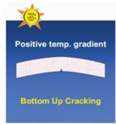
Figure 3.4.5. Critical load and structural response location for JPCP bottom-up transverse cracking.
